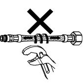
Never twist or stretch the flexible hose during installation.
